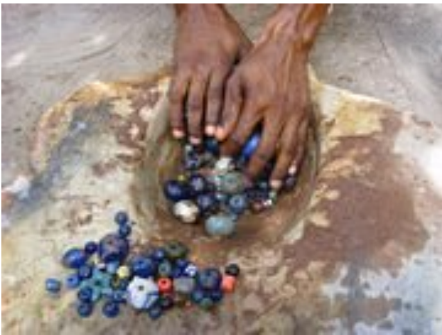
The last step consists in washing and polishing the beads by rubbing them forcefully
