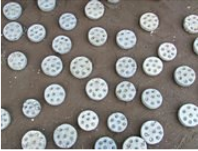
Beads are left to cool slowly in the moulds to prevent from cracking.
