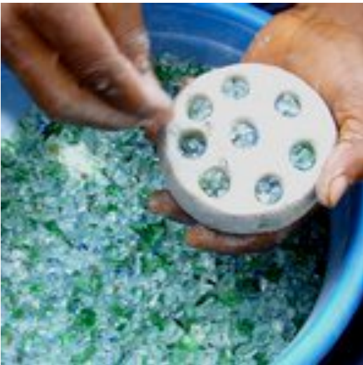
Filling of a mould with glass
